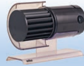
1971: Braun, Germany, HL70, designed by R. Weiss/J. Geubel, plastic, tangential impeller, blade diameter 60 mm
